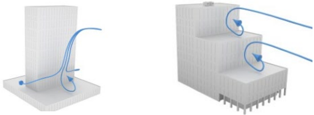
Image 2: Podium and tower setback for wind control
